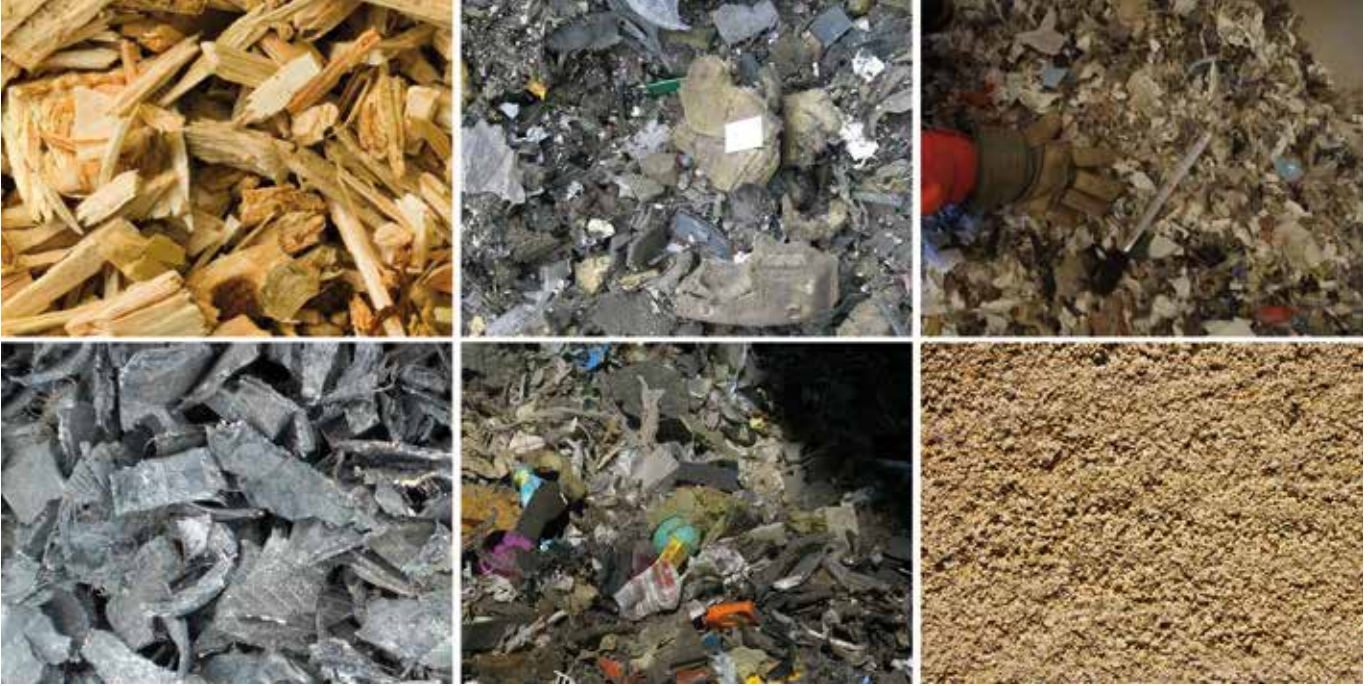
Figure 1: Examples of different fuels: wood chips, production waste, lightweight shredder fraction, shredded tires, recycled waste, waste dusts
